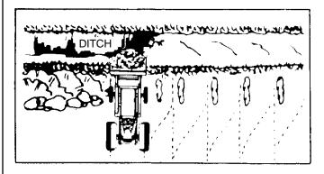
Leave dirt which drifts over the side of the bucket for final clean-up.
